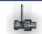
Configuration: Inline Segmented Body Thru port Pressure: 5000 PSI Nominal Size: 2 Inch Material Construction: 316 Stainless Steel (Bar) 1" and 2" Threaded / 1", 2" and 3" Flanged End Connections: Manual / Automated Operation: MultiStage Construction: 1 or 2 Stages Fluid Maintenance (WOG) **Design Function:** Oil / Gas Production and Injection Application: Location: Upstream gathering system
