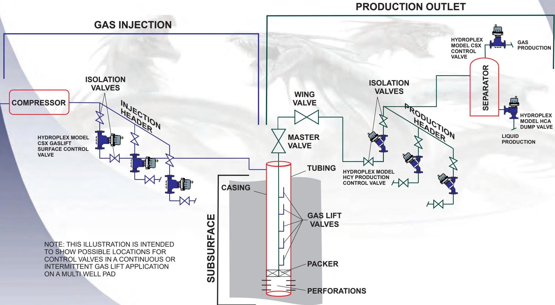
NOTE: THIS ILLUSTRATION IS INTENDED TO SHOW POSSIBLE LOCATIONS FOR CONTROL VALVES IN A CONTINUOUS OR INTERMITTENT GAS LIFT APPLICATION ON A MULTI WELL PAD
