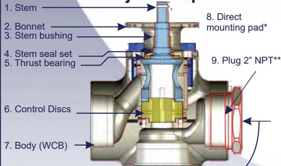
\*\*NOTE: Valve is configured as an angle body to convert to inline move plug as illustrated
